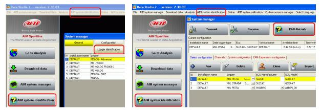
If all works correctly, "System identification/CAN-NET info" window, shown below, appears.
